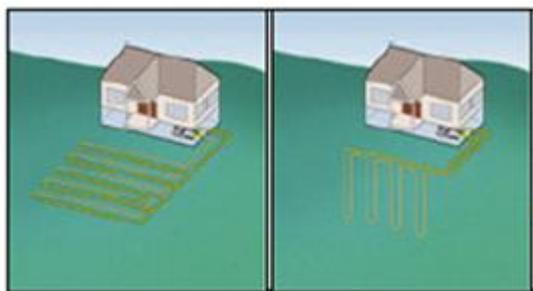
Horizontal Array    Vertical Boreholes
